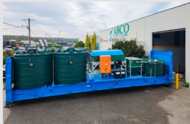
The portable mobile wastewater treatment system was built in Australia for rental purposes.
